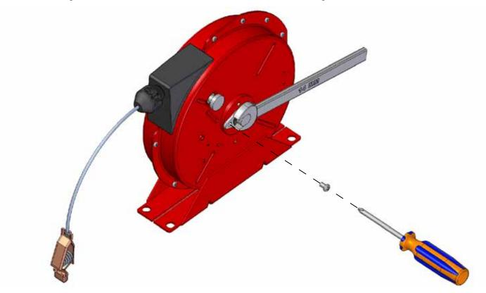
3. Using wrench, turn shaft counter-clock wise to decrease cable tension or turn shaft clock wise to increase cable tension.
