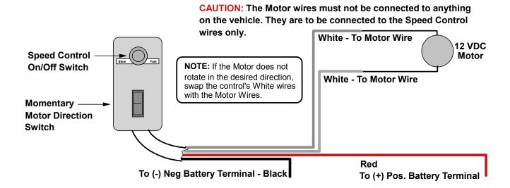
CAUTION: Do not connect the speed control Black wire to the positive battery terminal and do not connect the speed control Red wire to the negative battery terminal.
