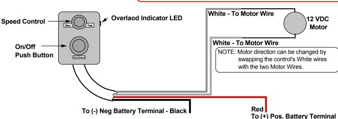
CAUTION: Do not connect the Black wire to the positive battery terminal and do not connect the Red wire to the negative battery terminal. This will cause a dead short condition across your battery terminals which will result in the circuit breaker tripping and will cause damage to the Speed / Switch Control unit. Do not use a motor direction, or reversing, switch on the Red and Black wires.
