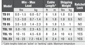
"Gable lengths listed are "active" or "working" cable. Maximum temperature 150 °F (65 °C).
